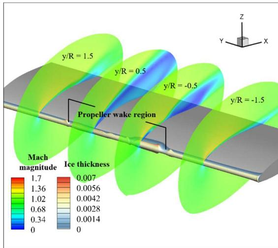
**Fig. 30** Separation occurrence through velocity contours at sectional positions of the propeller wake-induced iced wing.
