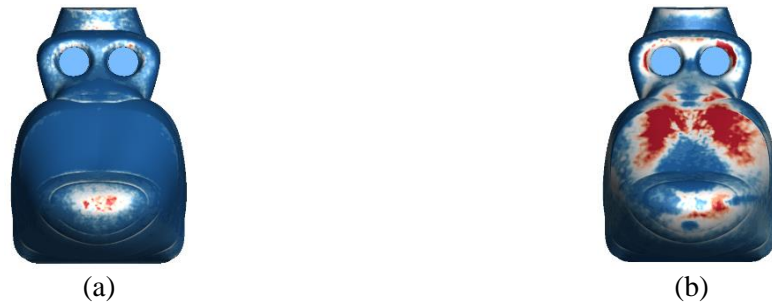
Fig. 27. Comparison of ice accretion between without rotor (a) and with rotor (b) at a high advance ratio.
