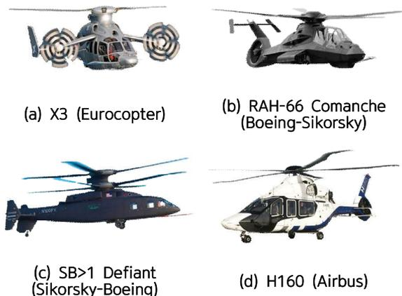
Fig. 1. Helicopters with hub fairing
