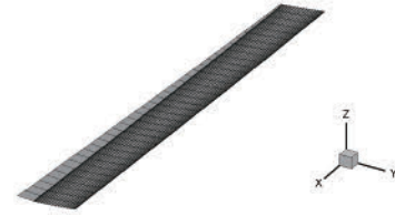
Fig. 5. Sharpe's rotor blade modeled by vortex lattice
