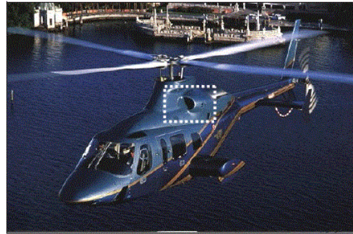
Bell 430: side mounted intake
