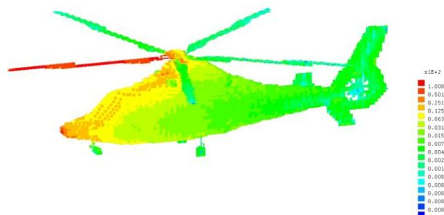
Fig. 11. Contour plot of the current density on the EC-155B surface.
