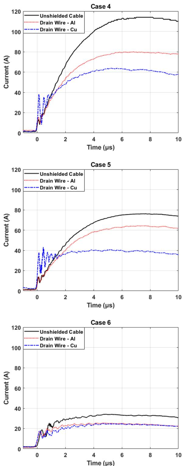
Fig. 7. Comparison of induced current at Waveform 1 and Level 5 condition: (a) case 4 with one cable; (b) case 5 with three cables; (c) case 6 with five cables.
