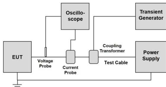
Fig. 3. Cable bundle test setup of DO-160.
