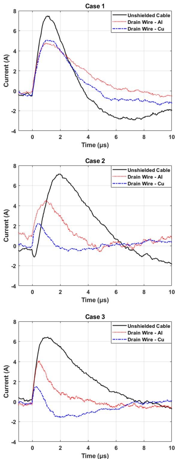
Fig. 6. Comparison of induced current at Waveform 1 and Level 3 condition: (a) case 1 with one cable; (b) case 2 with three cables; (c) case 3 with five cables.
