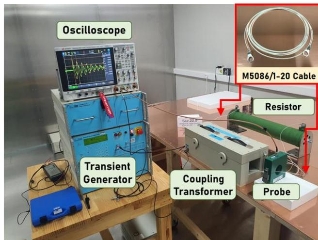
Fig. 4. Test setup for cable bundle test with M5086/1-20 cable.
