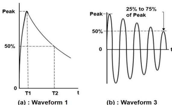
Fig. 1. Test waveforms 1 and 3 for the lightning indirect test.
