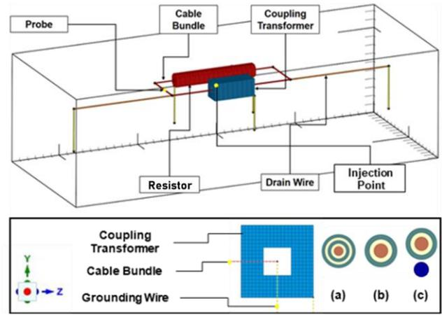
Fig. 8. Computational modeling of the cable bundle test.
