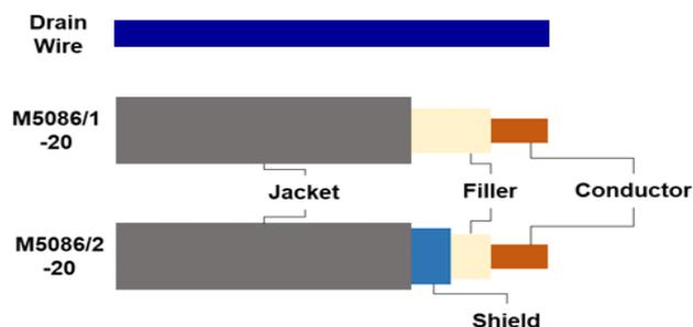
Fig. 2. Components of M5086/1-20, M5086/2-20 cables and drain wire.
