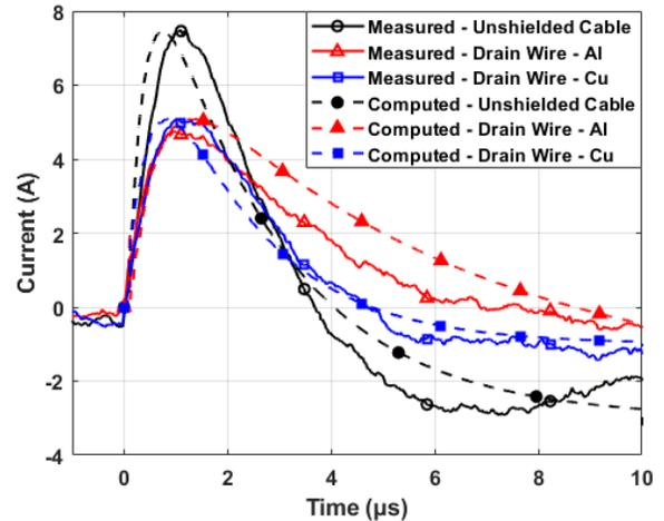
Fig. 9. Comparison of the test data and computational simulation results.
