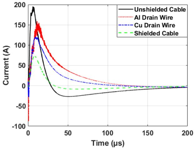
Fig. 12. Computational results of induced currents in unshielded cable, shielded cable, and cable with drain wire.
