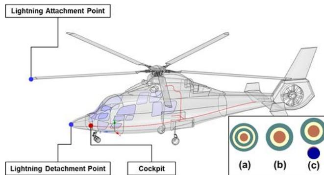
Fig. 10. Computational model of cable harness within EC-155B and cross-section of (a) shielded cable; (b) unshielded cable; and (c) cable with drain wire.
