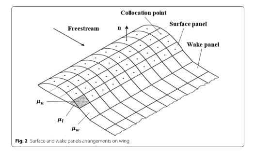
$$\sum_{k=1}^{N} \frac{1}{4\pi} \iint_{S_B} \mu \nabla \left(\frac{1}{r}\right) \cdot \mathbf{n} dS + \sum_{j=1}^{N_W} \frac{1}{4\pi} \iint_{S_W} \mu_W \nabla \left(\frac{1}{r}\right) \cdot \mathbf{n} dS - \sum_{k=1}^{N} \frac{1}{4\pi} \iint_{S_B} \sigma \left(\frac{1}{r}\right) dS = 0$$
