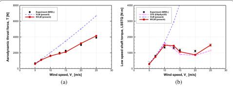
**Fig. 12** Comparison of rotor aerodynamic performance depending on wind speed: (a) aerodynamic thrust force and (b) low-speed shaft torque (LSSTQ)
