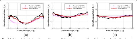
**Fig. 16** Azimuthal variation of normal force coefficient acting at specific radial positions for V = 10 m/s and  $\beta = 30^\circ$ : (a) r/R = 0.47, (b) r/R = 0.63, and (c) r/R = 0.8
