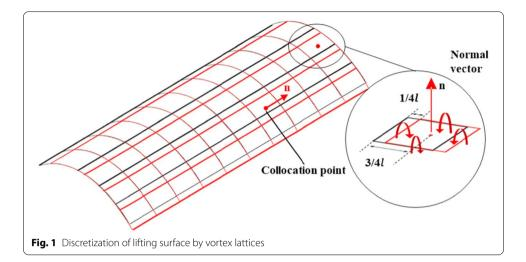
rotational velocity  $(\Omega \times r)$  at each collocation point.  $V_{\text{ind,bound,}}$  and  $V_{\text{ind,wake}}$  indicate the velocity components induced by the rotor blade and wake vortices.
