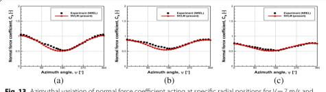
**Fig. 13** Azimuthal variation of normal force coefficient acting at specific radial positions for V = 7 m/s and  $\beta = 30^\circ$ : (a) r/R = 0.47, (b) r/R = 0.63, and (c) r/R = 0.8
