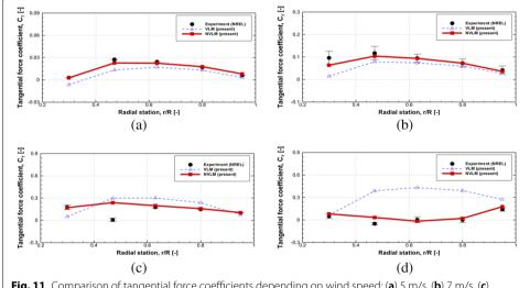
**Fig. 11** Comparison of tangential force coefficients depending on wind speed: **(a)** 5 m/s, **(b)** 7 m/s, **(c)** 10 m/s, and **(d)** 15 m/s
