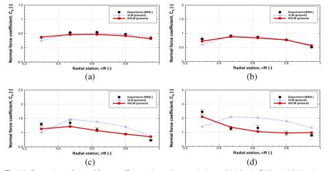
**Fig. 10** Comparison of normal force coefficients depending on wind speed: (a) 5 m/s, (b) 7 m/s, (c) 10 m/s, and (d) 15 m/s
