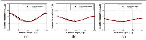
**Fig. 14** Azimuthal variation of tangential force coefficient acting at specific radial positions for V = 7 m/s and  $\beta = 30^\circ$ : (a) r/R = 0.47, (b) r/R = 0.63, and (c) r/R = 0.8
