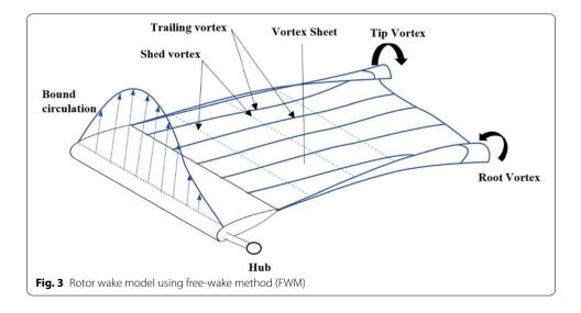
the previous time step. Once the wake vortices are shed, their strengths remain constant according to Helmholtz's theorem.
