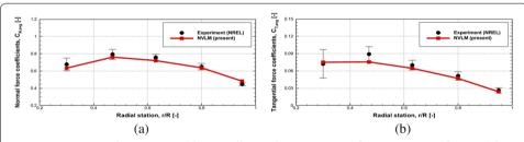
**Fig. 15** Comparison of time-averaged force coefficients for V = 7 m/s and  $\beta = 30^{\circ}$ : (a) normal force and (b) tangential force coefficients
