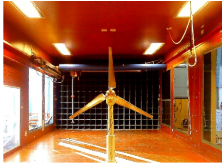
Fig. 11. Closed-loop wind tunnel facility in NTNU and scaled-down wind turbine model [26]
