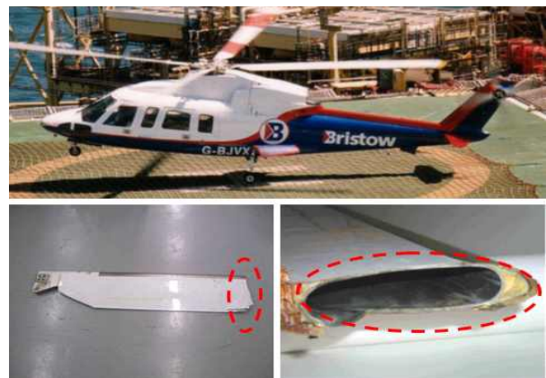
Fig. 1 Lightning strike accident (Sikorsky S-76A+).
