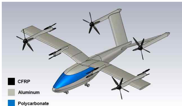
Fig. 7 Model of UAM aircraft implemented in simulation.
