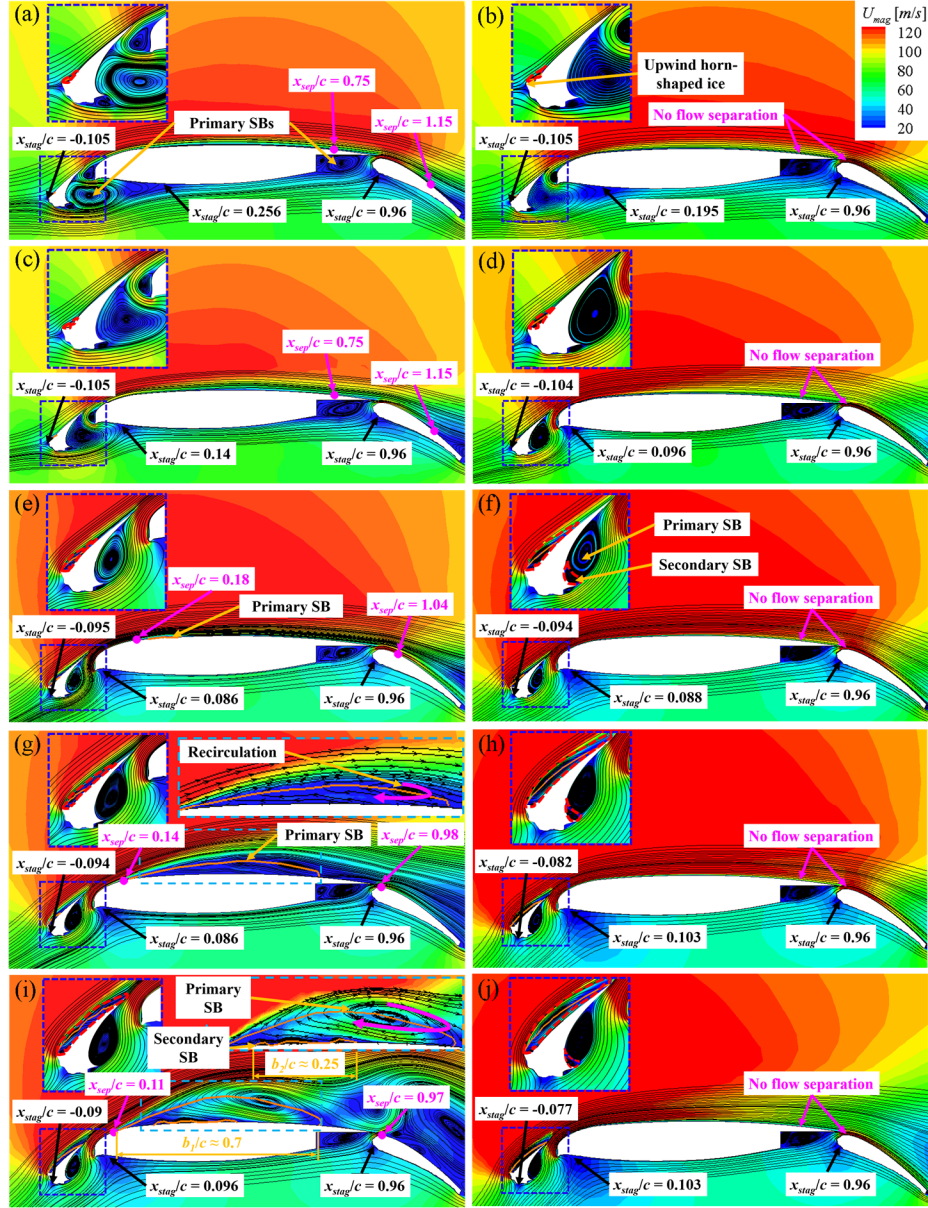
Fig. 14 Identical to those in Fig. 12, but for non-SLD case. Solid orange lines denote the mean stagnation lines generated by primary and secondary SBs on upper surfaces of slat and main elements.
