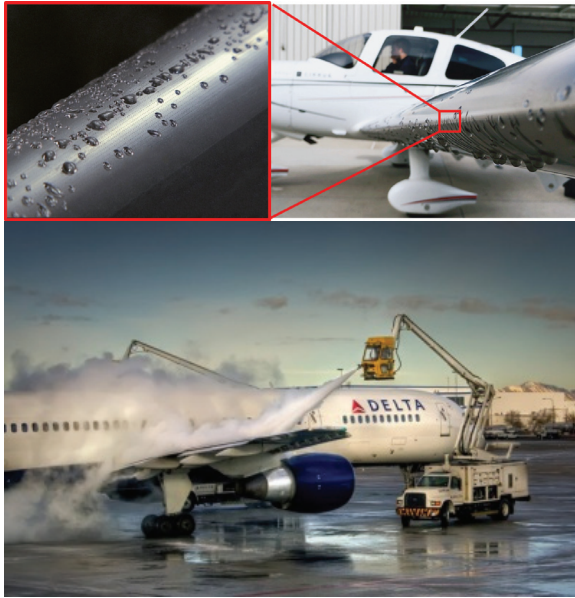
Fig. 4. Fluid protection system (top) and de-icing before takeoff (bottom)
