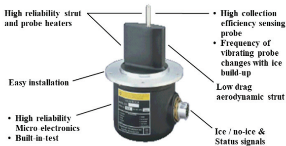
Fig. 12. Configuration of vibrating probe ice detector (Rosemount Aerospace Inc.)
