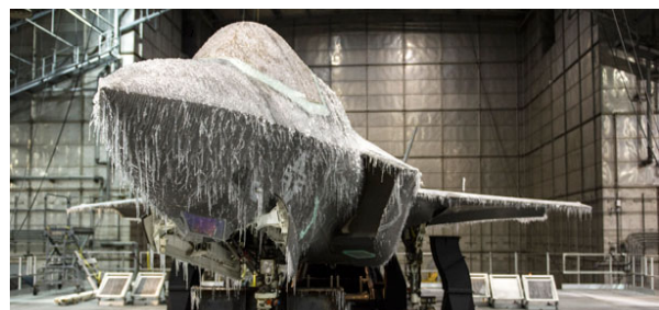
Fig. 6. Full frame icing/freezing rain on F-35 [12]
