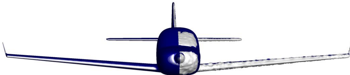
Figure 7-18 SLD ice accretion on the KC-100 aircraft
