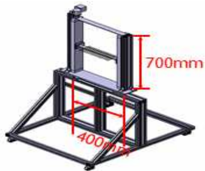
Fig. 5. Detailed description of temperature measuring device
