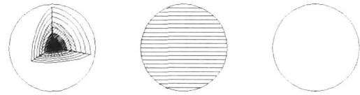
Fig. 1. Simulated ice hail composition. Spherically layered(left); flat-wised layered (center); monolithic layered (right).
