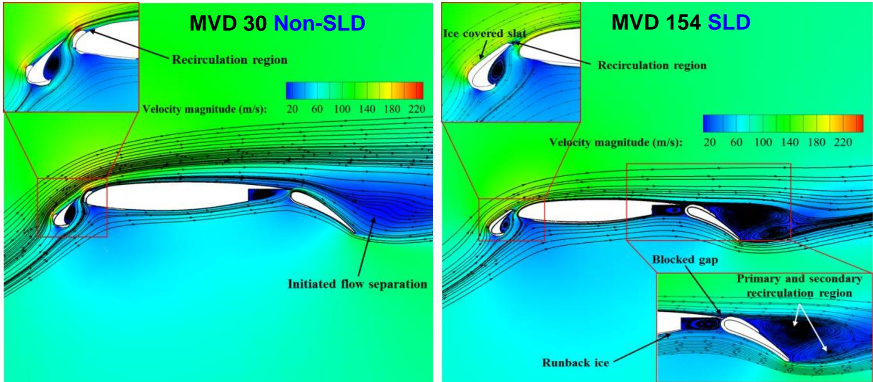
**No leading edge ice formed on the suction side of the main element for the SLD condition,** leading to a significant reduction in loss of performance. This runs **counter to previous studies on iced single element airfoils**, in which the aerodynamic performance loss was higher for SLD icing conditions.
