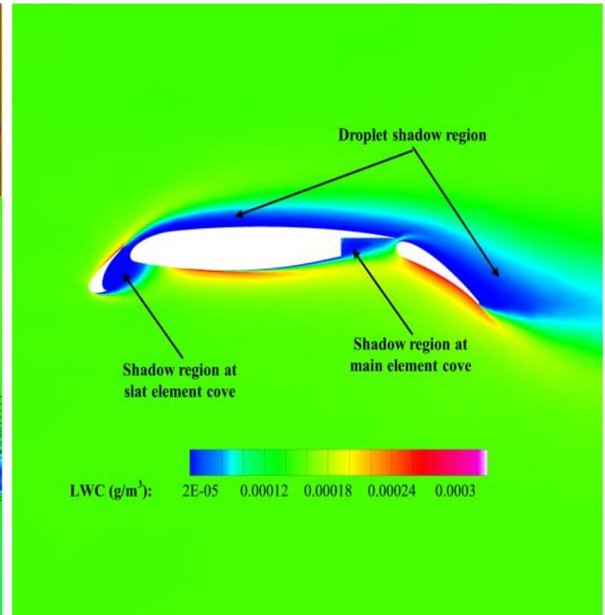
**Very complicated flow-fields:** Improper modeling of droplet could easily result in a numerical breakdown due to the strong circulation and flow separations on the slat and the main element cove.
