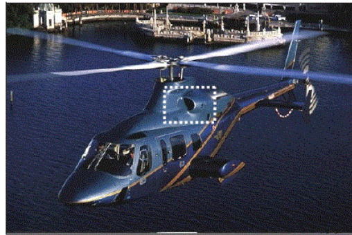
Bell 430: side mounted intake
